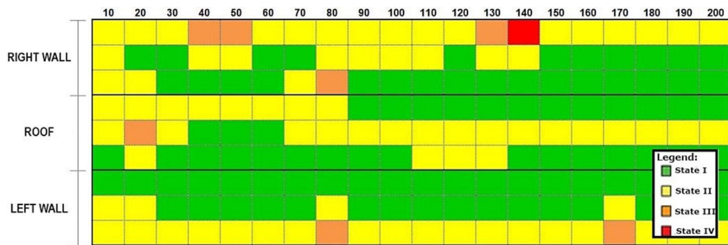
(3) Inspection data in grid deterioration classification
