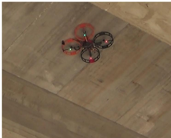
Figure 2-13 Prototype of multirotor system operating in contact with the ceiling. [144]
