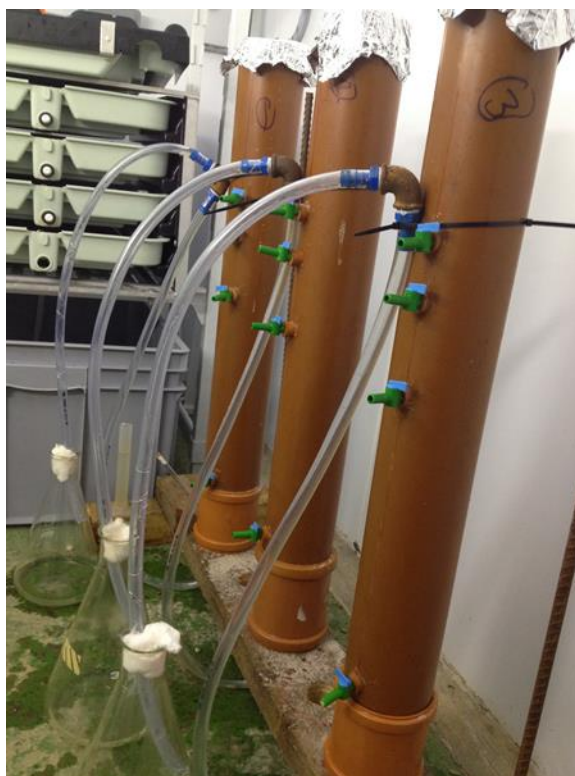
Figure 5.2: Photograph of the bench-scale filters using in the study.
