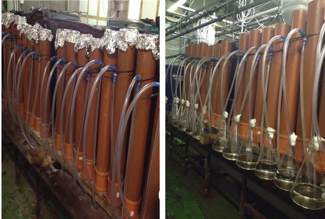
Figure 4.2: Bench-scale biosand filters used in the study with different resting water depths.
