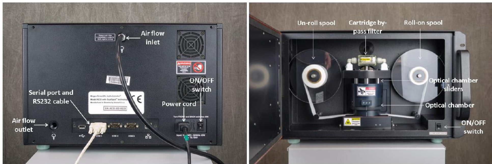
Figure 2.1. Rear view of the model AE33 aethalometer (left) and inside view of the instrument from the front (right), with labels of relevant components (NOAA, 2016).
