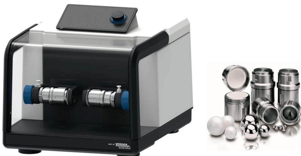
Figure 1-4: Laboratory-scale ball mill (MM 400, Retsch, Haan, Germany). The stainless-steel milling jars are mounted onto the milling unit and secured using blue locking wheels. On the right, the interior of the milling jars is shown, along with the milling balls. The white balls are made of zirconium oxide, while the others are composed of stainless steel.
