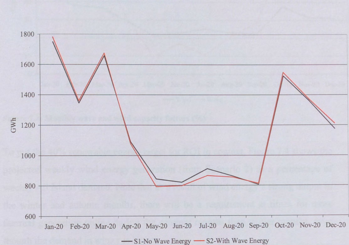
Figure 7.2: Monthly wind (S1) and wind and wave generation (S2) (GWh) for target year. Scenario 1 is shown in black for wind only-scenario. Scenario 2 is shown in a red line for wave and wind combination.
