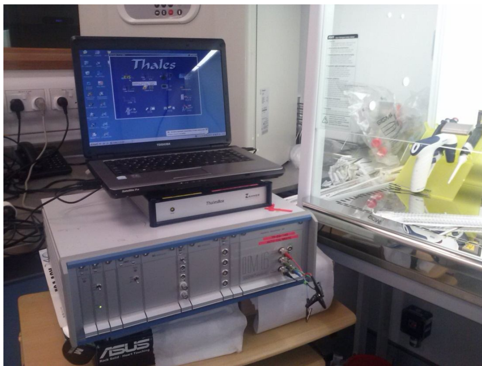
Figure 3.1: Zahner impedance analyser setup near the fume hood for cytotoxicity measurements
