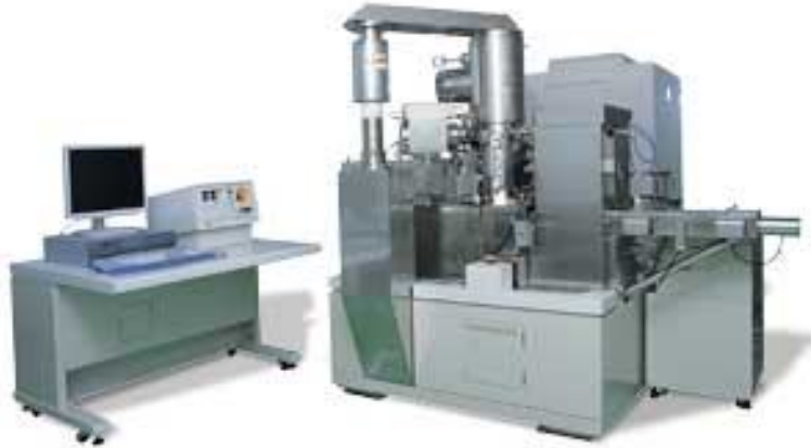
Figure 1.14: Jeol 6000FS/E Electron Lithography System available in Tyndall National Institute.
