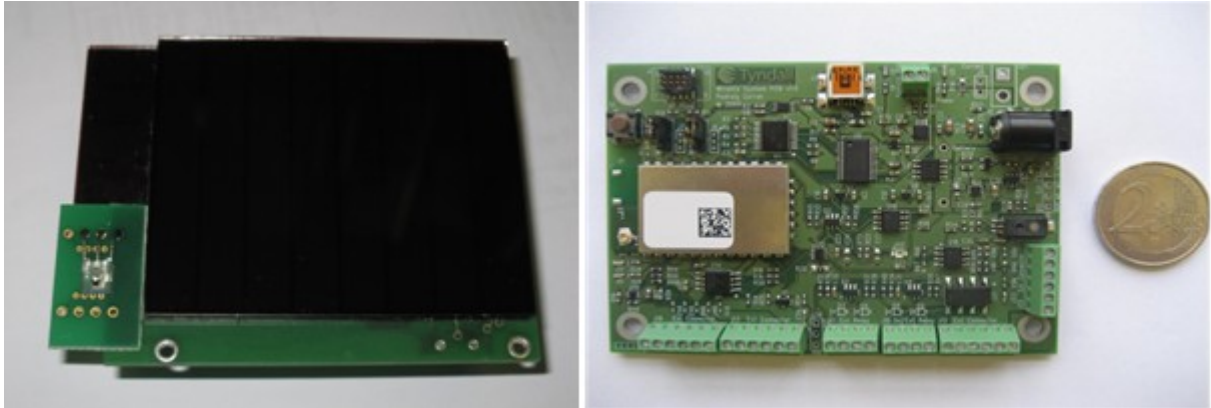
Figure 6. Implemented Indoor Light Powered WSN with Hybrid Energy Storage Compared to capacitive energy storage [1], the proposed hybrid energy storage solution reduces the average leakage current by 45% to 12.5 \mu\text{A} . The effective capacity of the energy storage is also increased 25% to 1.3 mAh.
