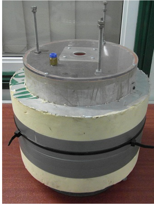
FIG. 1. A generic cylinder OWC wave energy converter.
