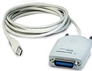
Figure 3.3: Agilent 82357a USB-to-GPIB converter used in this thesis.
