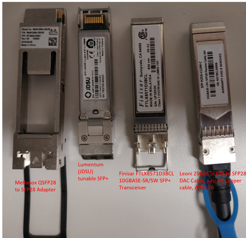
Figure 4.12: Transceivers, Mellanox adapter and components used for connection between Tofino switch, Lumentum ROADM and Spirent packet tester.
