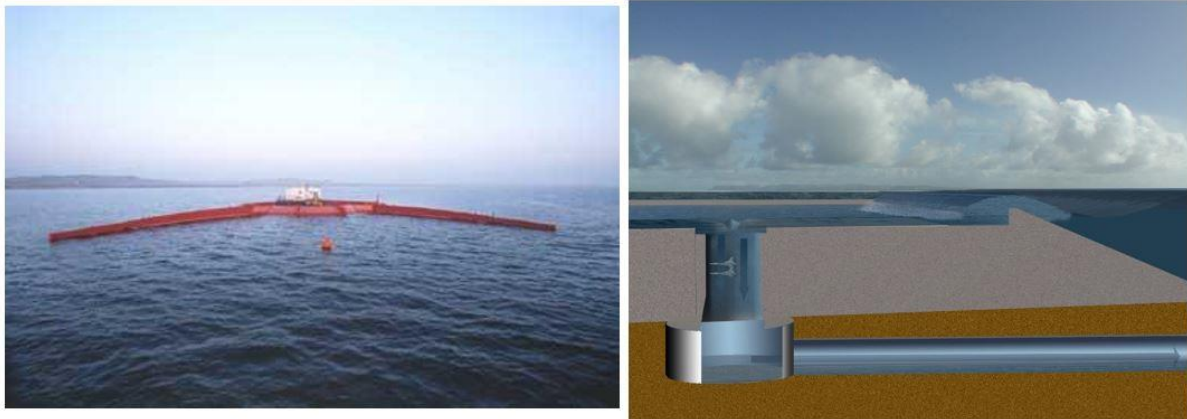
Figure 2.10 The figure on the left hand side shows the WaveDragon device (Tethys, 2021). The figure on the right hand side shows an example of an overtopping device (Aquaret, 2012).
