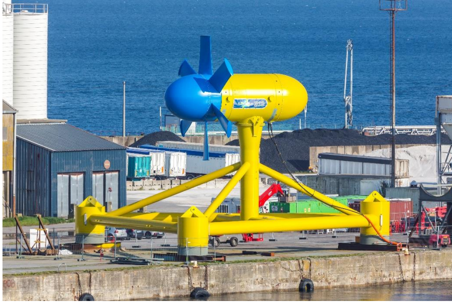
Figure 2.20 Sabella D10 Horizontal axis turbine (Sabella, 2021).
