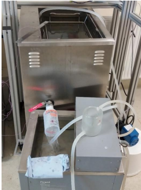
Figure 3-1. The setup for ultrasound treatment using the water bath system.
