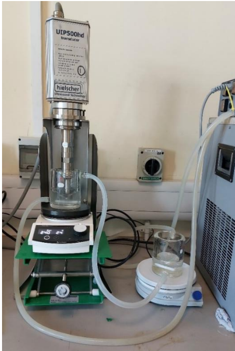
Figure 4-1. The setup for ultrasound treatment using the probe system.
