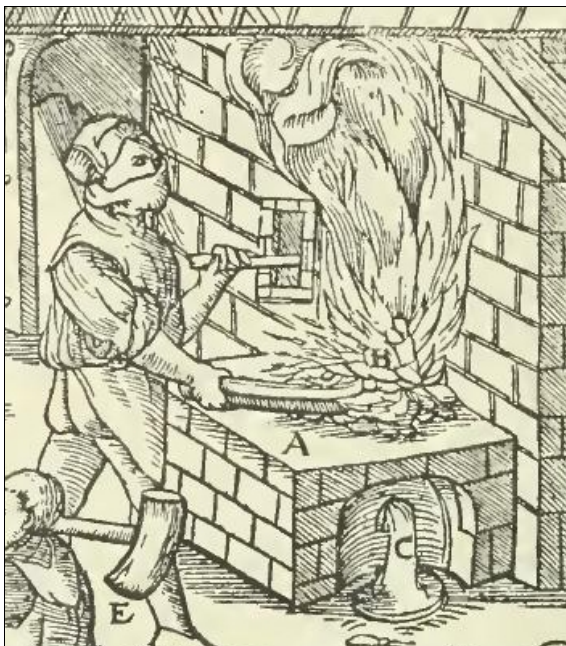
Fig. 3.3 Water-powered open hearth furnace, Bohemia, mid-16 th century (Agricola et al. 1912 [1556]: 421)
