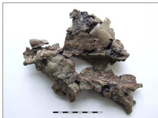
Fig. 6.9 Smelting slag, Ballykilmore, Co. Westmeath (scale: 100mm) (Young 2012c: 420)
