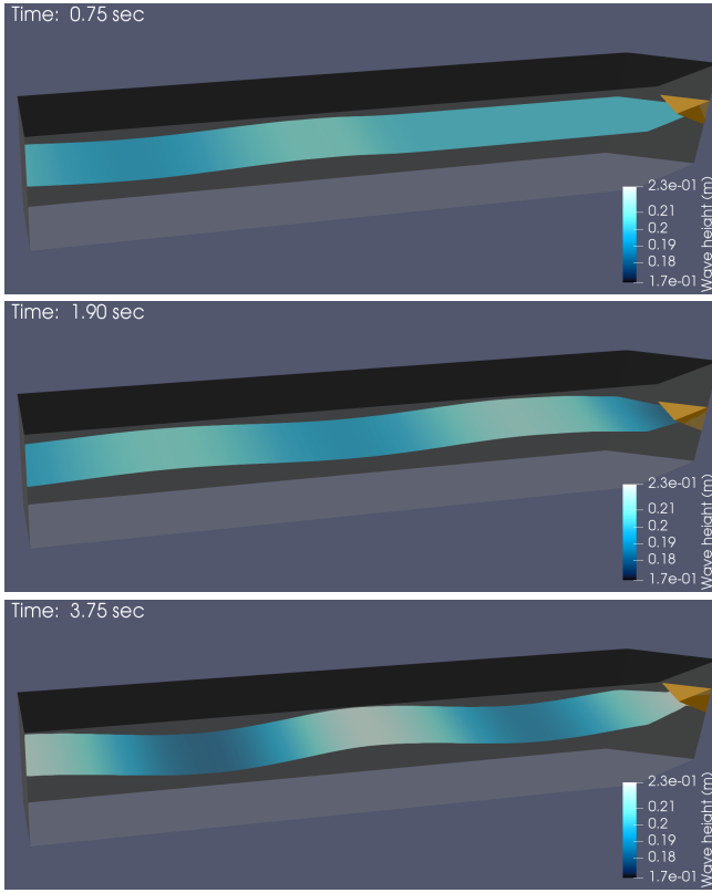
Fig. 4. Snapshots of the numerically computed free surface h(x, y, t) = \bar{H}(x, y) + \eta(x, y, t) (colour denotes height in meters, with initial still water level H_0 = 0.2\text{m} ), as it evolves in the wavetank with V-shaped contraction (times shown on the pictures). The buoy resides in the corner of the contraction and is shown using orange colour.
