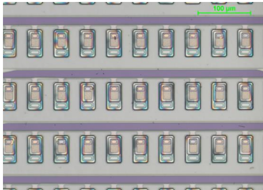
(b) After release etch in 5% TMAH
