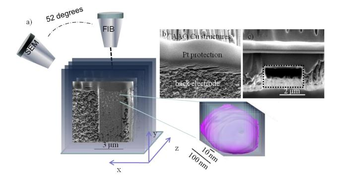
Figure 1. a) Schematics of the serial sectioning FIB/SEM nano-tomography method, b) tilt view SEM image of the AAO/Cu nanostructures before commencing serial sectioning featuring continuous Au back electrode and Pt protection, c) Ga-ion beam image of the same area after serial sectioning showing milled away volume of material starting from the back electrode with the corresponding markers for correction of the drift on the ion-beam column.
