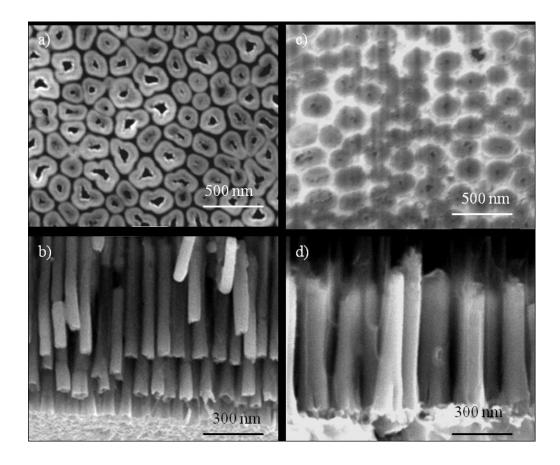
Figure 2. Plan view SEM images of Cu nanostructures embedded within AAO for a) sample A and c) sample B, and cross-sectional views obtain after cutting the samples in two for b) sample A and d) sample B.
