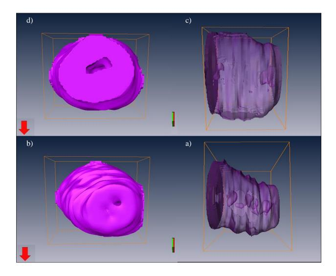
Figure 5. 3D reconstructions for two different Cu nanostructures (upper and bottom rows) corresponding to sample B. Two visual representations of one and the same nanostructure are shown a) and c) in solid color, and b) and c) transparent and rotated by 90 degrees. The surrounding AAO matrix is omitted for clarity.
