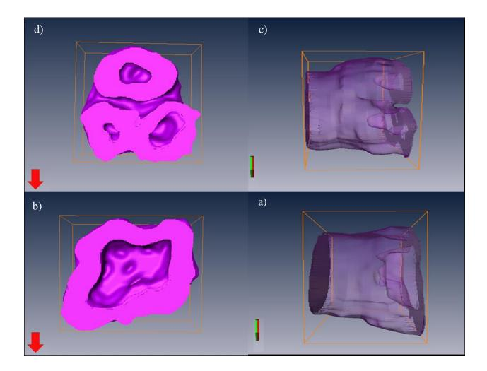
Figure 4. 3D reconstructions for two different Cu nanostructures (upper and bottom rows) corresponding to sample A. Two visual representations of one and the same nanostructure are shown a) and c) in solid color, and b) and c) transparent and rotated by 90 degrees. The surrounding AAO matrix is omitted for clarity.
