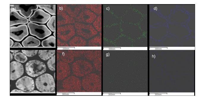
Figure 6. STEM HAADF images for a) sample A and e) sample B whereas the thin foils are extracted from areas at about 150-200 nm away from the back electrode, b) and f) the corresponding EDX Cu mapps, c) and g) the corresponding EDX Al maps and d) and h) the corresponding EDX Au maps.
