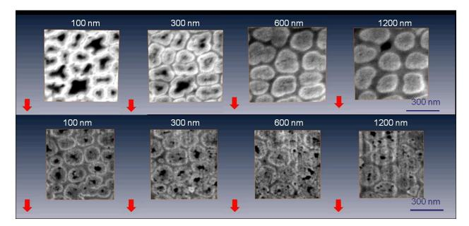
Figure 3 Series of plan view SEM images taken at four different lengths from the back electrode obtain after sequential FIB milling. The upper and bottom rows correspond to sample A and B.
