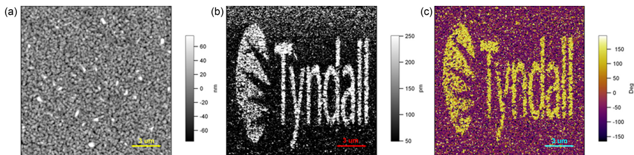
FIG. 11. Images of BTF7M3O on SiO 2 -Si: (a) topography, (b) out-of-plane PFM amplitude, and (c) out-of-plane PFM phase after PFM lithography with an applied dc bias of 33.0 V.
