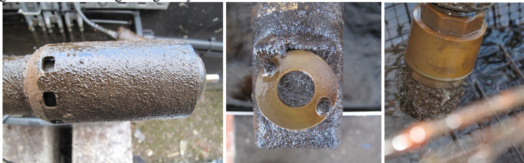
Figure 3. Biofouling associated with estuarine conditions on standard sensors
