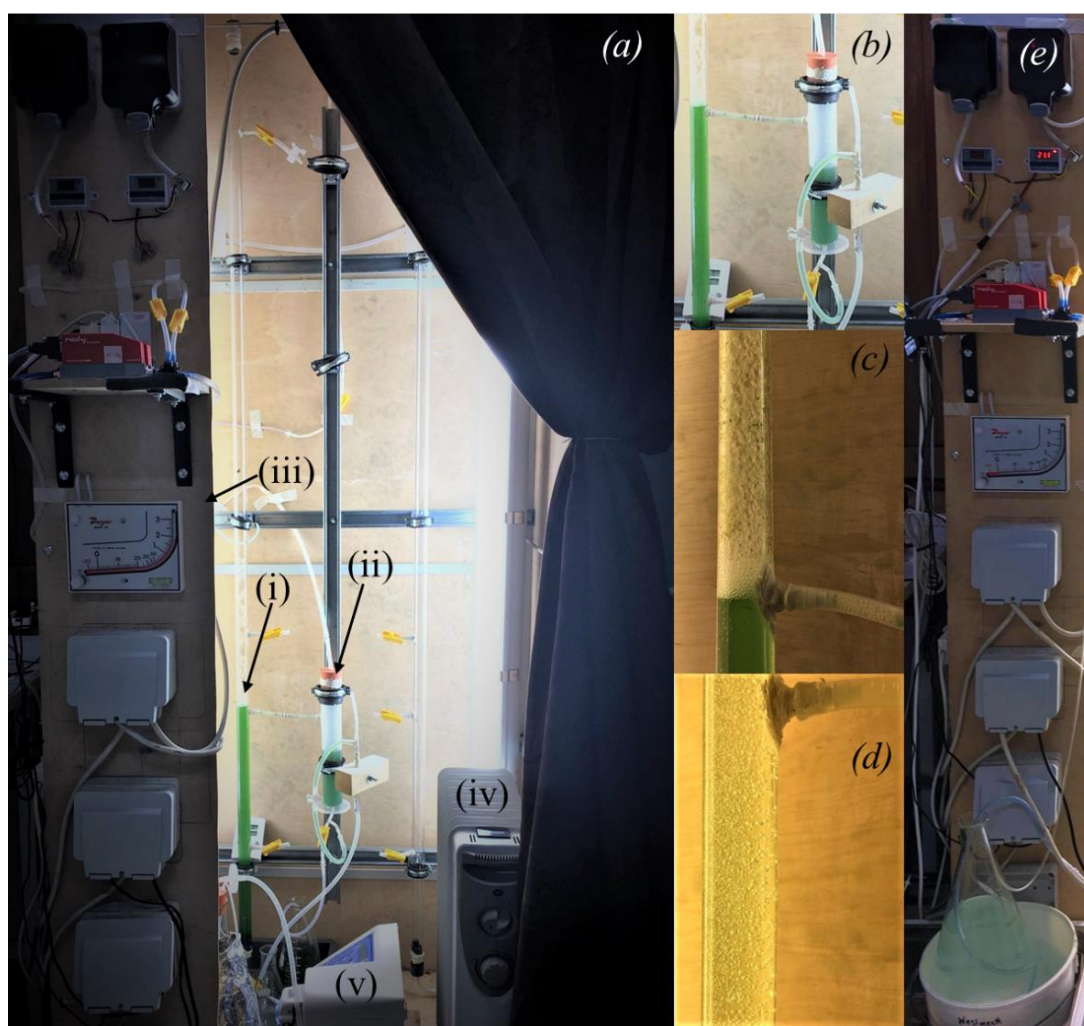
Figure 3-2 Pictorial representation of the experimental setup for photosynthetic biogas upgrading with (a) the overall bubble column reactor setup within a temperature and light controlled housing; (b) detail of the gas-liquid separator with a U-loop to prevent emptying by syphoning and also adjust the outlet liquid flow rate as per the inlet flow rate; (c) example of foaming observed during operation with high algae concentration; (d) representation of homogeneous flow regime characterised by uniform bubble size under low algal concentration; and (e) detail of the control panel with the condensate trap placed within an ice bath (bottom of the figure). Additional details marked in figure (a) represent (i) the bubble column (additional tapping points for future experiments); (ii) the gas-liquid separator; (iii) control panel with gas flow controllers, mass flow meter, manometer gauge, and the switches for temperature control; (iv) the heater; and (v) the peristaltic pump
