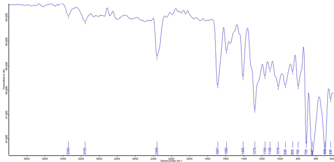
Figure 1: IR Analysis for a 1:1 mixture of INA: BA analysed after 1 minute of milling in the Retsch MM400 mixer mill
