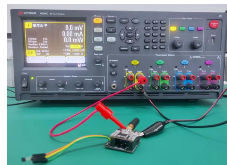
Fig. 16. Test setup for WSN module power consumption measurement.
