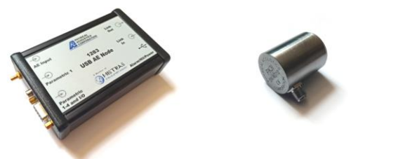
Fig. 1. AE monitoring system - flow-chart (top), Physical Acoustics data acquisition device (bottom left) and AE sensor (bottom right).
