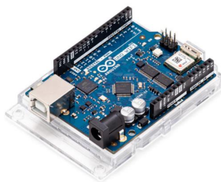
Figure 4. 23 Arduino Uno WiFi Rev2 (20)
