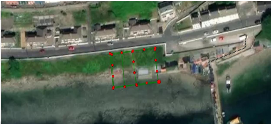
Figure 4. 21 Photogrammetry points collected by the drone
