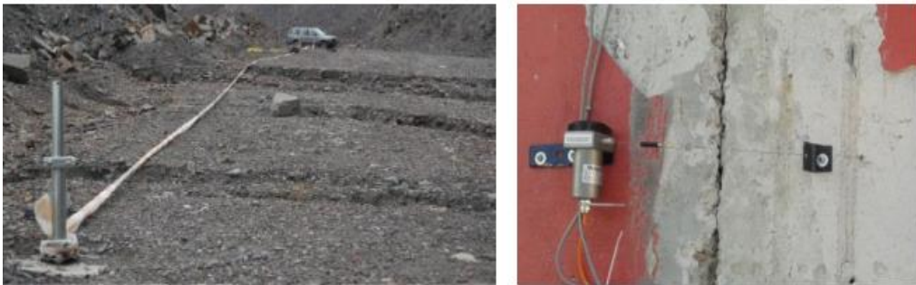
Figure 3. 8 Extensometer in action (10)
