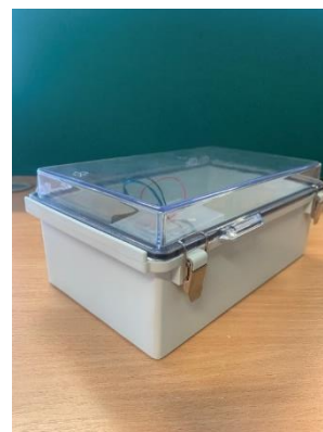
Figure 4.37 Waterproof sensor case
