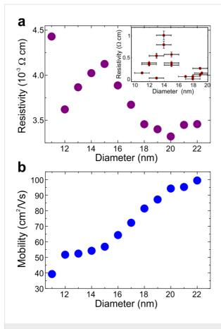
**Figure 3:** (a) Calculated nanowire resistivity from 22 to 11 nm diameter. Around 14 nm a peak-feature is found in agreement with the experimental data. At 11 nm diameter, the sharp increase of the resistivity is due to the shift of the Fermi-energy below the third heavy-hole sub-band (Supporting Information File 1). (b) Nanowire mobility calculated for the same diameter range as in (a). After an initial decrease, the mobility reveals a plateau-like region from about 12 to 15 nm.
