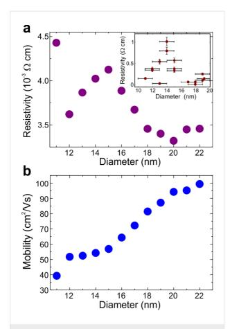
Figure 3: (a) Calculated nanowire resistivity from 22 to 11 nm diameter. Around 14 nm a peak-feature is found in agreement with the experimental data. At 11 nm diameter, the sharp increase of the resistivity is due to the shift of the Fermi-energy below the third heavy-hole sub-band (Supporting Information File 1). (b) Nanowire mobility calculated for the same diameter range as in (a). After an initial decrease, the mobility reveals a plateau-like region from about 12 to 15 nm.
