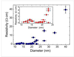
Figure 1: Resistivity of nanowires with 40 to 11 nm diameter. The resistivity decreases by two orders of magnitude with reducing diameter. In the range of 27 to 20 nm an increased scattering of the resistivity values is observed. Below 20 nm the resistivity variation is significantly smaller. Inset: Data for NWs with diameter below 25 nm. At around 14 nm a peak-like feature is found.
