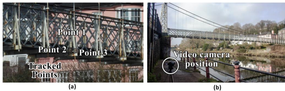
Figure 6 (a) Tracked points at the centre of the span used in video based analysis, and (b) Position of the video camera in relation to the bridge.
