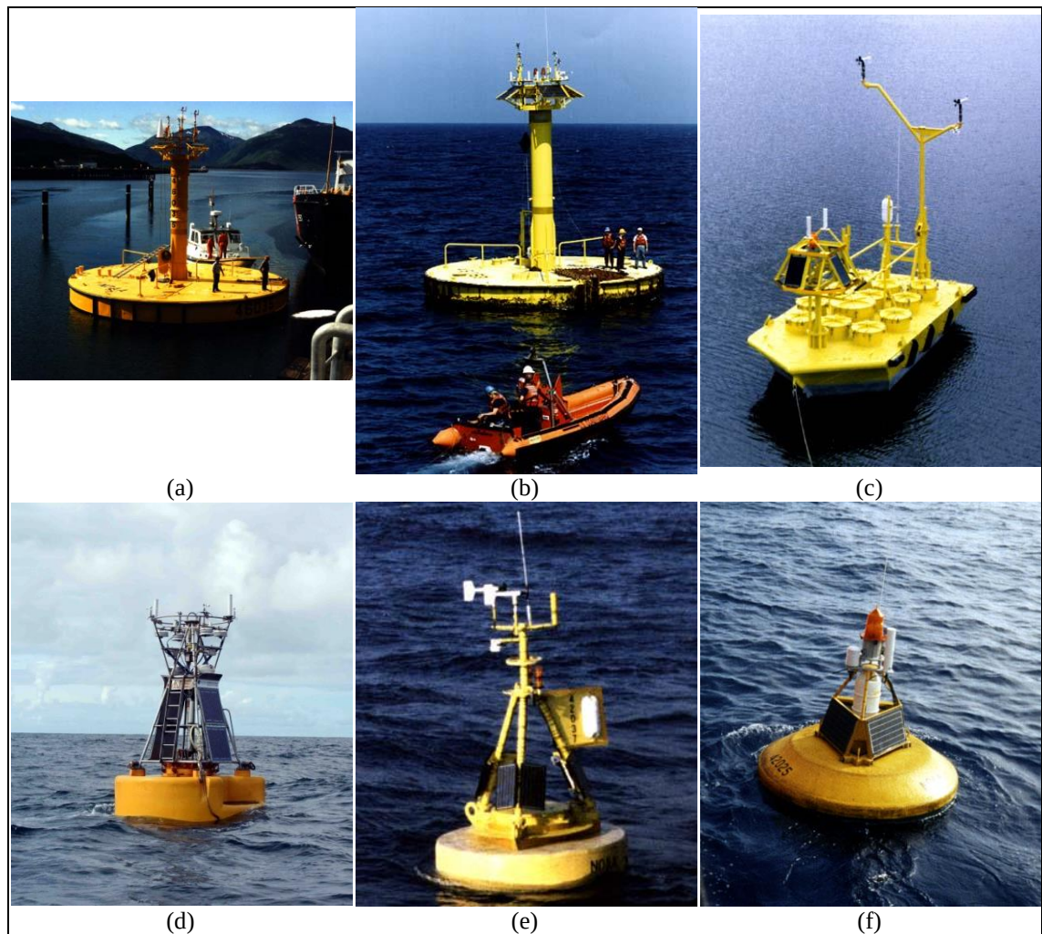
Figure 2.3. ODAS hull types.
