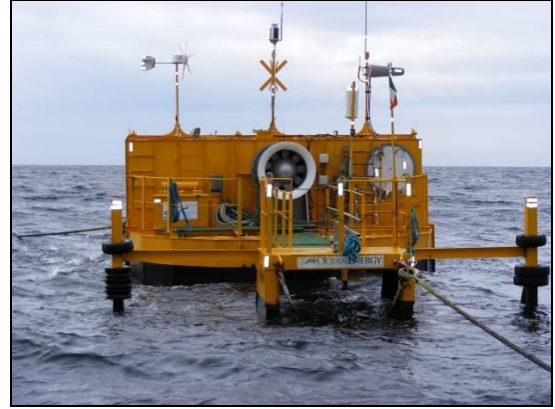
Figure 2. Scaled Air Turbine on the OE Buoy.
