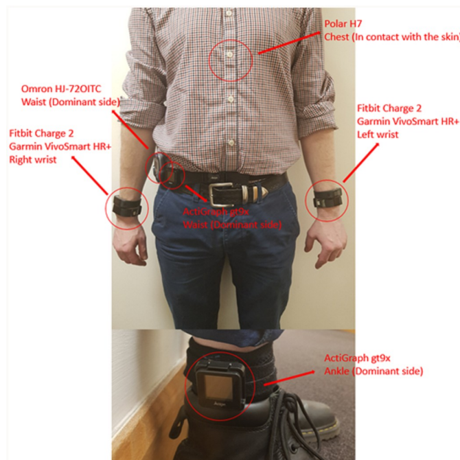
Fig 1. Devices positioning. Polar H7, Fitbit Charge 2, Garmin VivoSmart HR+, ActiGraph GT9X-BT, Omron HJ-720ITC. Philips Health Watch and Withings Pulse Ox are not illustrated in the picture but are worn in the same position of the Fitbit and Garmin devices.
