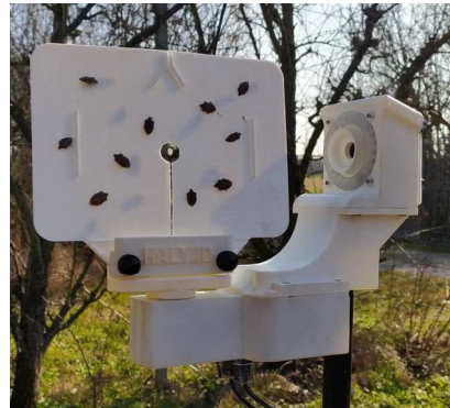
Fig. 1. Deployed device in an orchard for dataset collection from a sticky double-sided trap.
