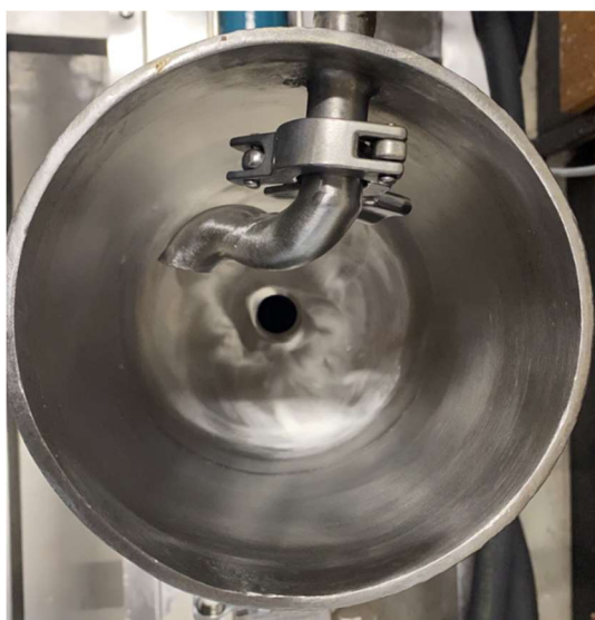
Figure 1.4.: Top down view of the feed vessel from the modified fouling rig set-up, showing the feed tube designed to return product at an angle to promote turbulence without aeration or foaming.
