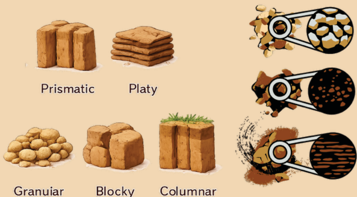
Figure 5. Common types of soil structure: granular, blocky, platy, prismatic, and massive. AI-generated image (OpenAI/ChatGPT, 2025), edited by Caroline Delpupo using Canva® (Canva Pty Ltd., 2025).
