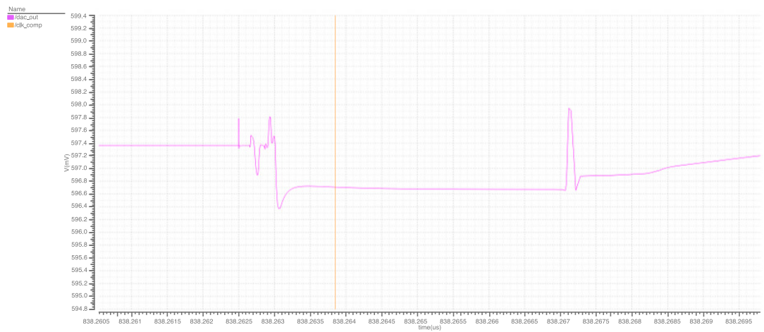
Figure 3.27: Comparator being enabled after DAC settling.
