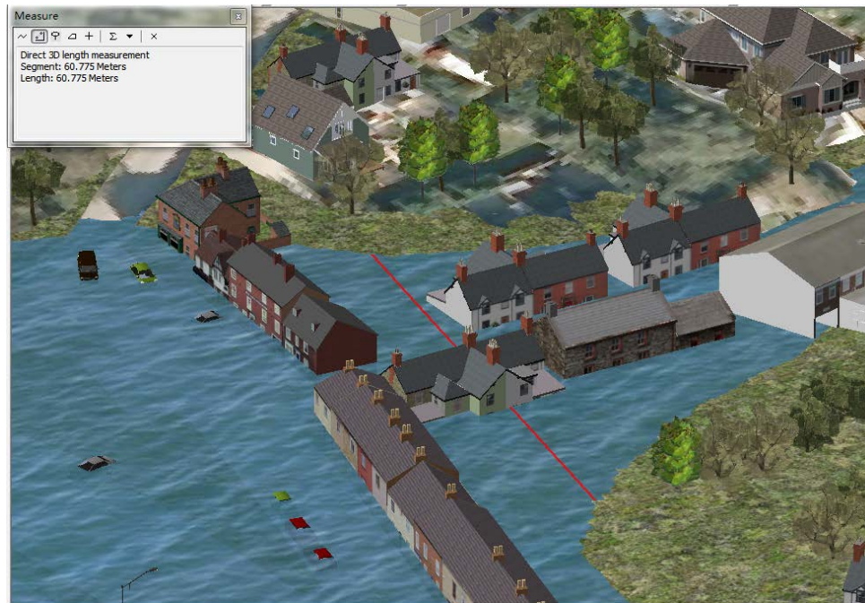
Figure 7.11 Spatial distance measurement. This screen snapshot shows the 3D length measurement function provided in ArcScene.
