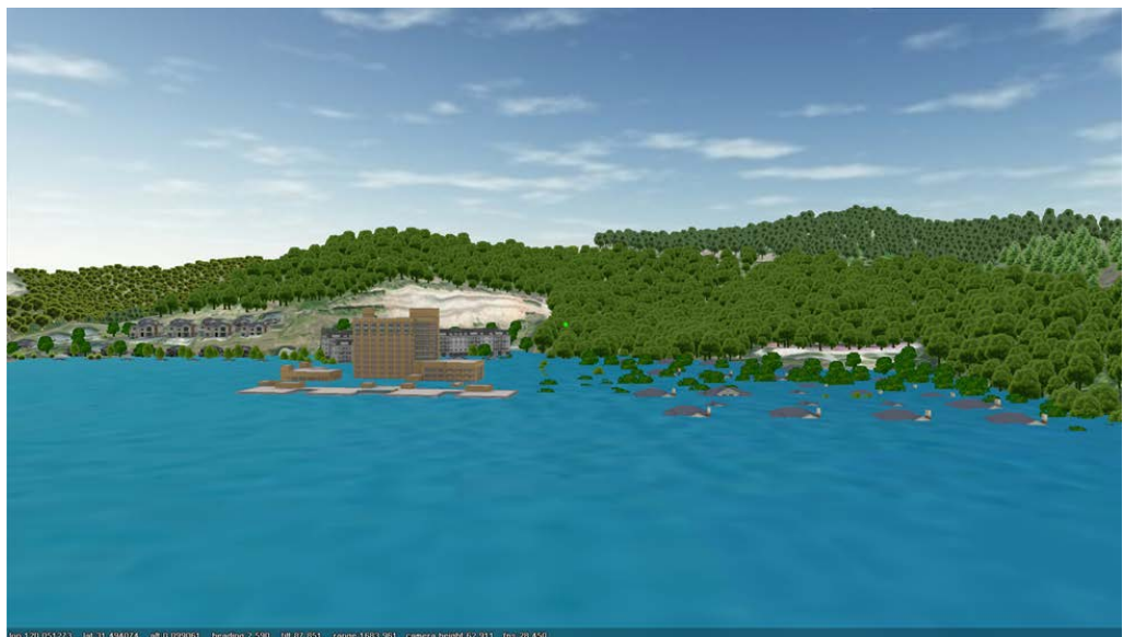
Figure 7.29c Water level can be set to extreme values. In this screen snapshot, the water level is set to 15m which is unlikely to happen in the real world.
