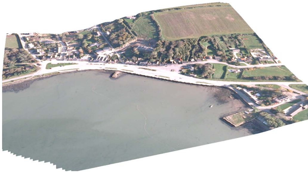
Figure 7.6 Mashup of the high-resolution DEM and the aerial imagery of the site. The aerial imagery is elevated using the height information contained in the DEM.
