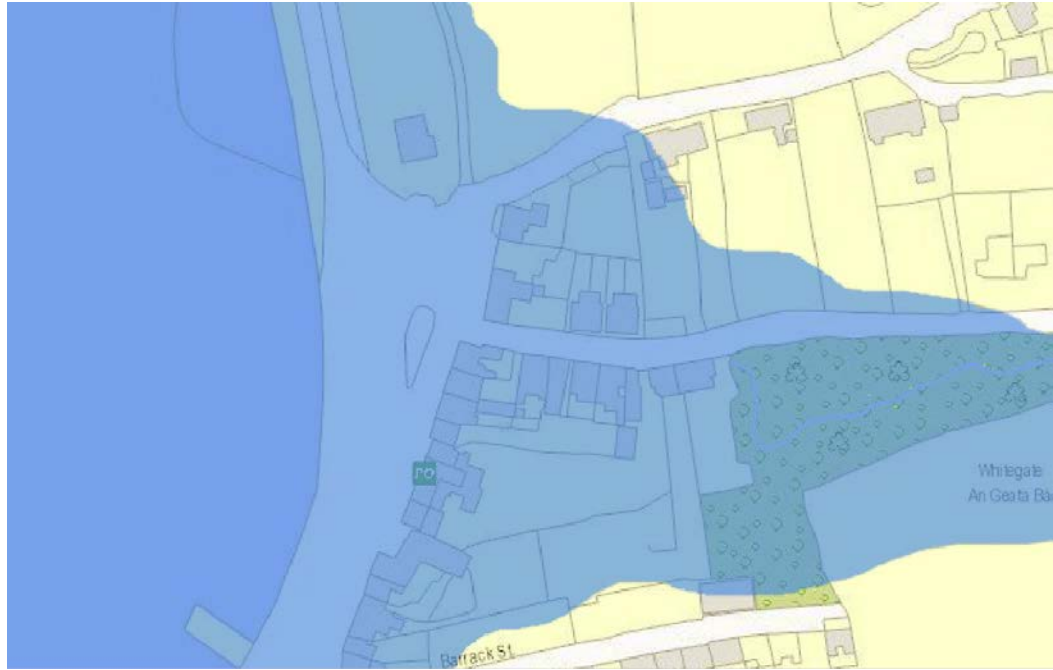
Figure 7.12 Quick mashup of 1:4000 Bing Map. This screen snapshot shows a basic topographic map overlapped with a blue color layer to show the flooded zone.
