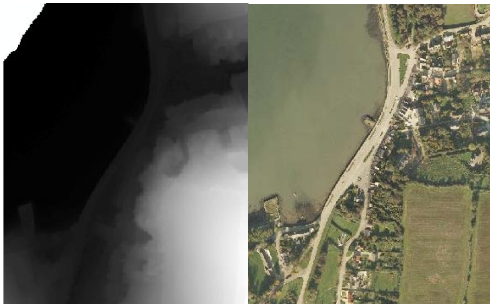
Figure 7.4 DEM and aerial photograph for Whitegate extracted from original data. The grey scale (black-white) indicates the change of elevation. The aerial photograph provides a high-resolution bird's view of the ground features such as roads, buildings, trees and fields.
