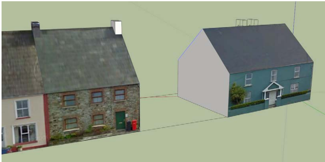
Figure 4.4 Creating 3D models in SketchUp using photographs captured on site
