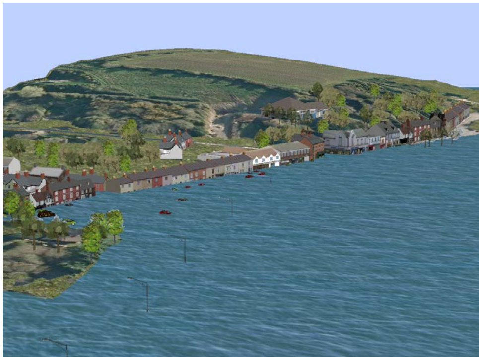
Figure 7.9 3D coastal inundation mapping for Whitegate (face south). The screen snapshot shows the scenario where the main roads in the town are flooded. The buildings next to the roads were all affected.
