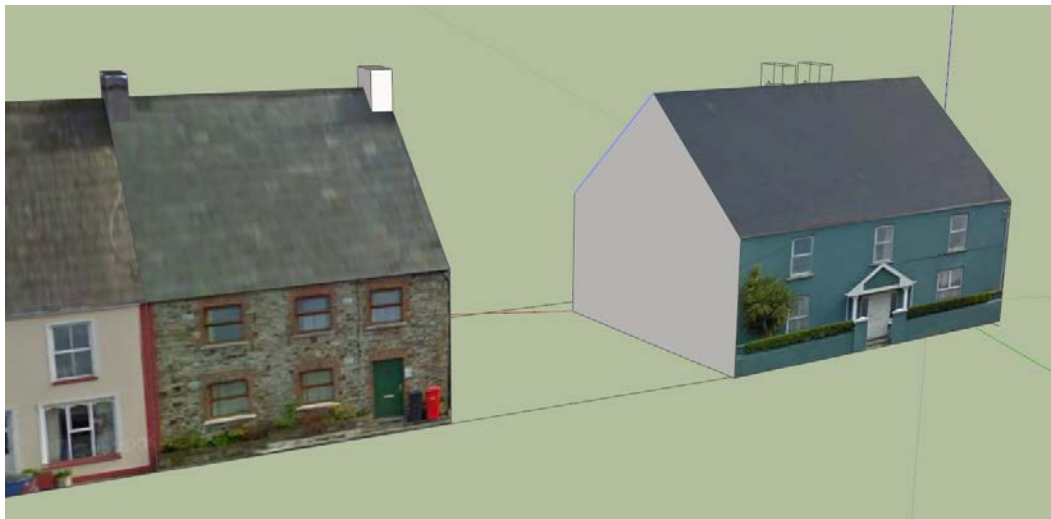
Figure 7.8b 3D building model creation in Google SketchUp 8. The texture is derived from the field photograph.
