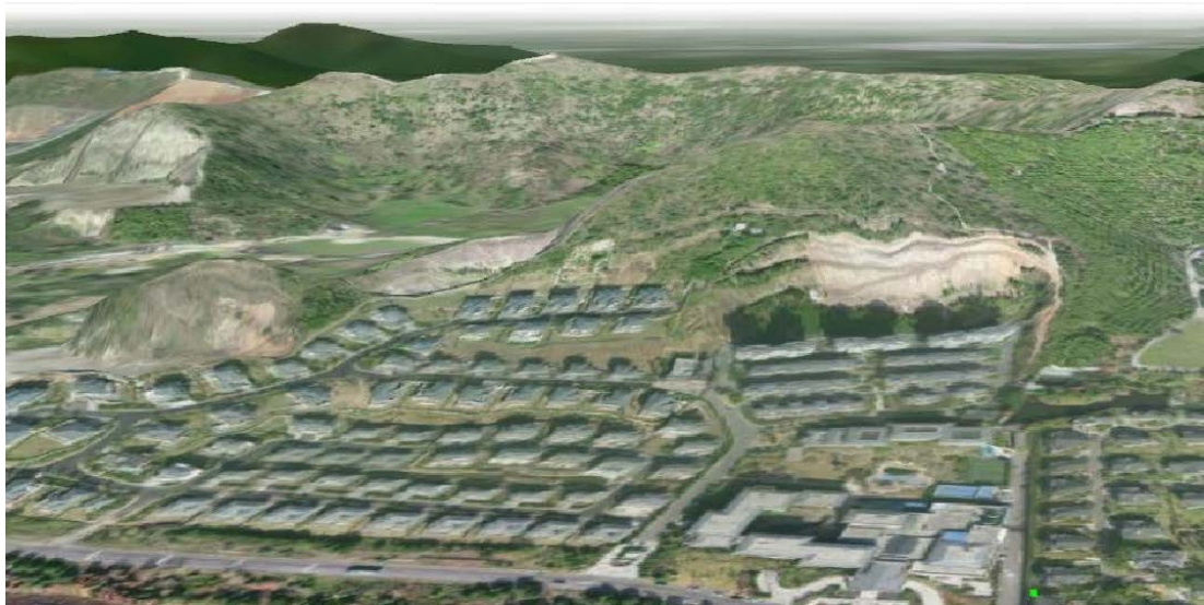
Figure 7.21 Basic terrain surface created by DEM (face north). This screen snapshot shows the elevated aerial photograph with support of high-resolution DEM. All the ground features are clearly viewed in this scene.
