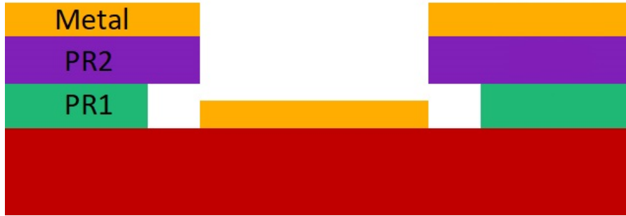
Figure 3.17: Schematic of the metal lift-off resist layout
