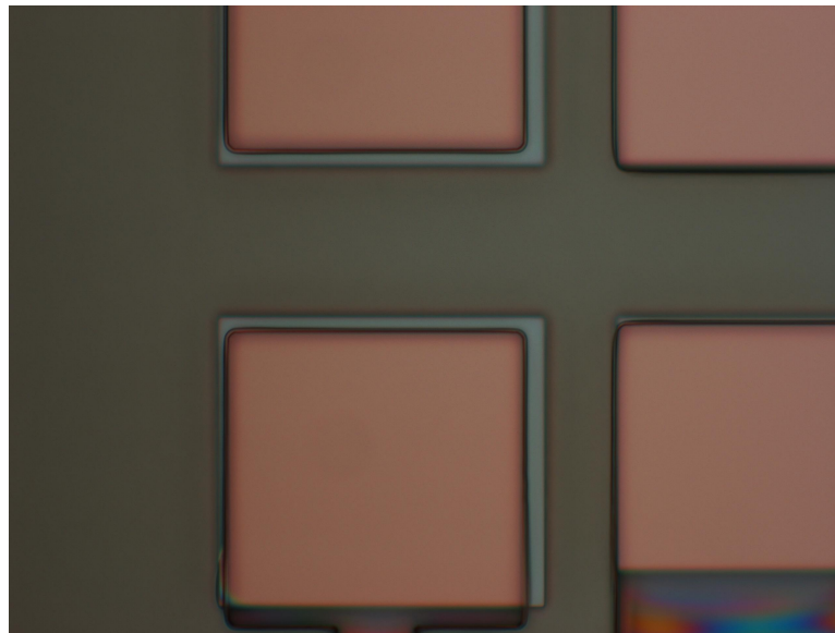
Figure 3.15: Microscope image of undercut photoresist on contact pads - the undercut is visible as the double line on the edges of the opening
