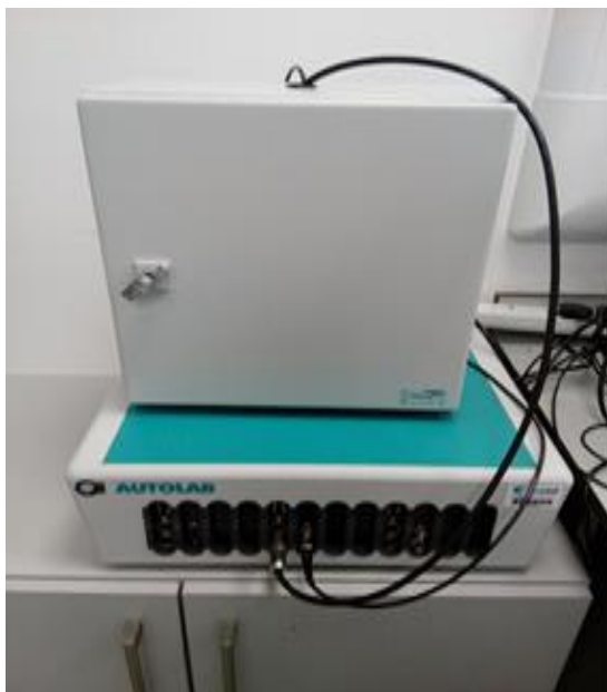
Figure 2.20: Laboratory based benchtop potentiostat, the Autolab PGSTAT302N and a Faraday cage.
