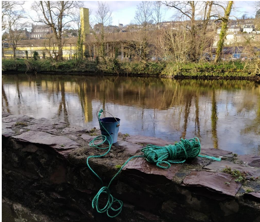
Figure 4.15: Water retrieval apparatus at site of water sample at River Lee Maltings, Cork.
