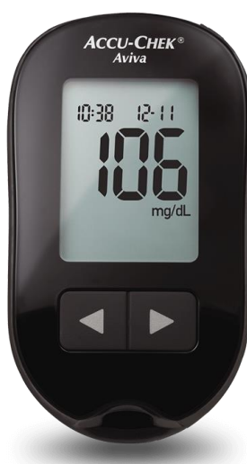
Figure 3.4: Roche Accu-Chek, which utilises the ADuCM350.
