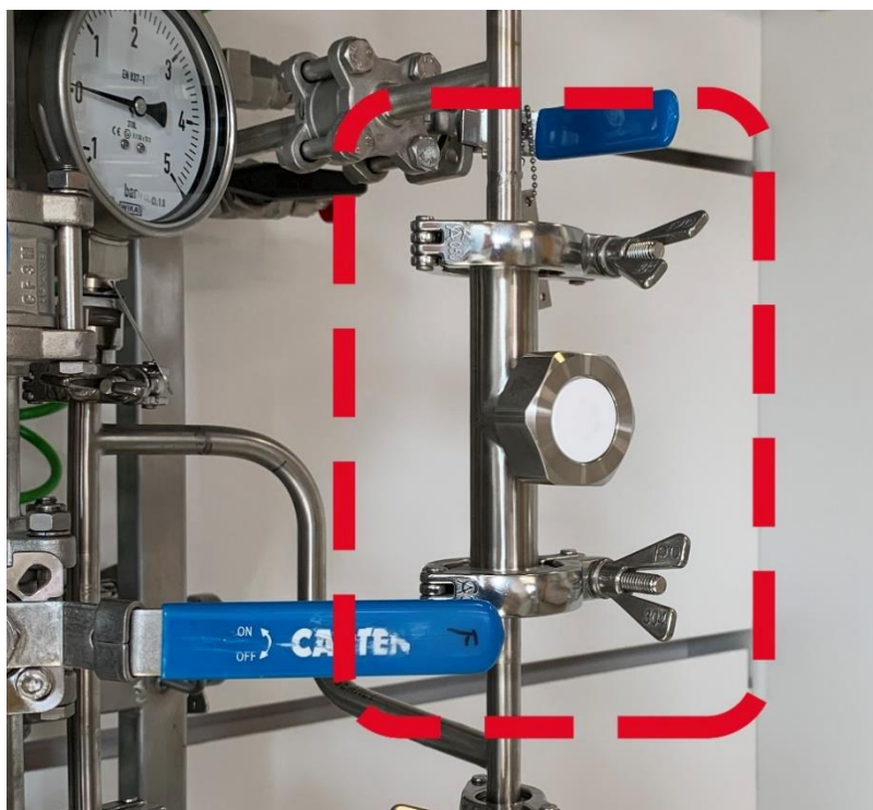
Figure 28: Gas Sampling port with sampling septum inserted located on the BHM rig. Above and below the sampling port are tri-clamps.
