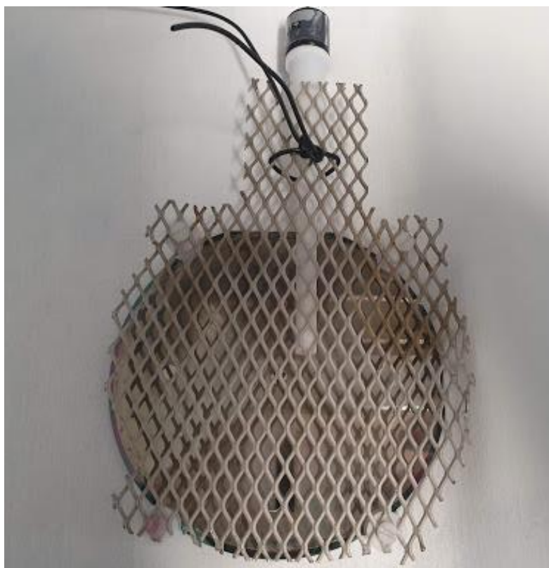
Figure 50 - Metal oxidations set-up: Pt/Ti mesh with Teflon holders securing a wafer. Hg/HgO electrode held between the wafer and mesh
