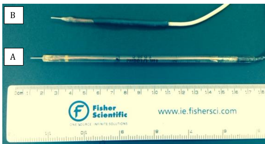
Figure 8.1 Handmade self-sealing platinum electrode made following the design reported by Topcu et al. (2008) (A) and made in our laboratory (B).
