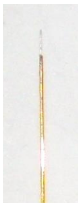
Figure 8.2 Schematic representation of the microelectrode electrode ( www.wpionc.com ) (A), picture of the electrode (B) and microscope picture of the tip of the electrode (C).
