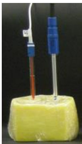
Figure 8.3 Measurement of redox potential in Cheddar cheeses. Silver/silver chloride reference electrode (red electrode) placed in a hole wide filled with 3 M KCl to complete the salt bridge with the working electrode that was inserted directly into the cheese.
