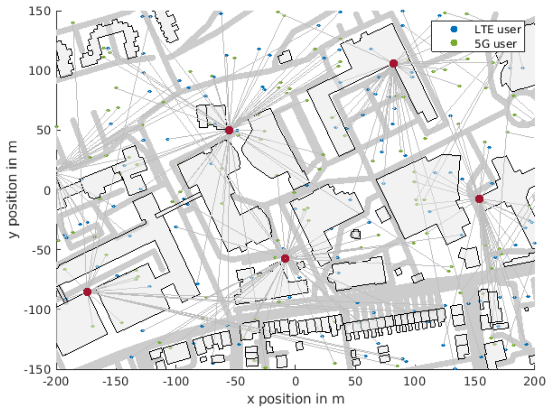
Figure 5.4: Figure illustrates a simulated urban network deployment showing the coexistence of 5G and LTE technologies. The red dots represent base stations (BS), while green and blue dots denote 5G and LTE users, respectively, connected to their nearest base stations, as indicated by gray connectivity lines
