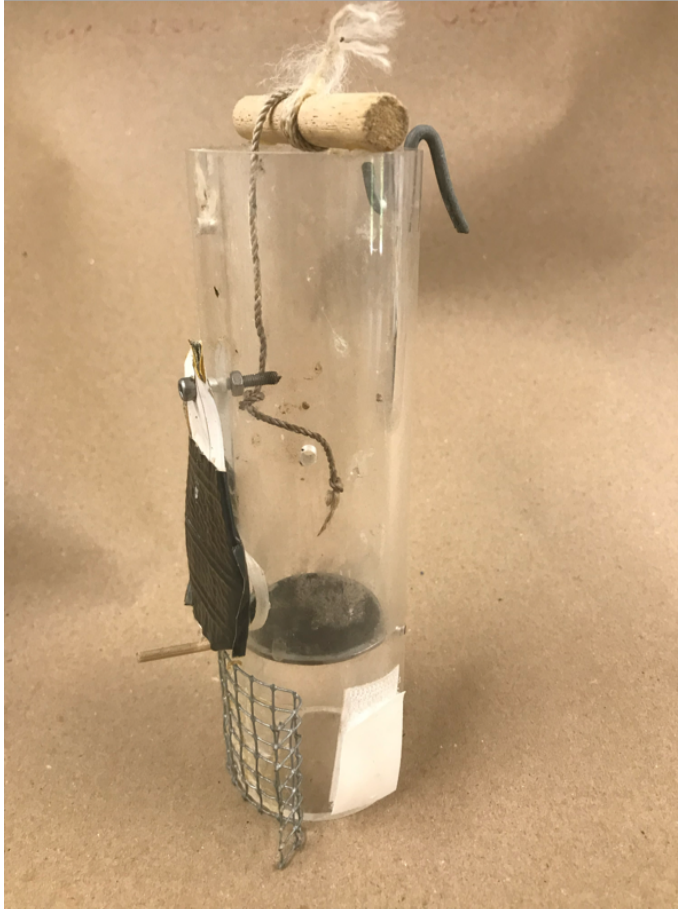
Figure S8. Problem solving device. Device can be solved by removing string through the top, opening the side door or removing the trigger to drop the platform.
