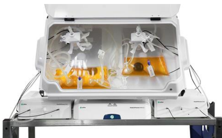
Figure 9: Single-use wave bioreactor bags for cell culture (Cytiva, n.d.).
