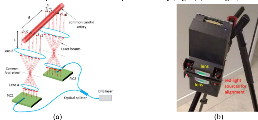
Fig. 1. (a) The 2 \times 6 LDV device with confocal lens systems, where s = 5\text{ mm} , d \geq 25\text{ mm} , L = 75\text{ mm} . (b) A picture of the 2 \times 6 LDV system. The two front lenses and four red-light sources for alignment can be seen.
