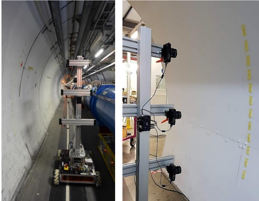
Figure 36 - illustration of the CERNbot mobile platform in addition to the depiction of the three-tier camera setup on the platform ( (CERN, n.d.)
