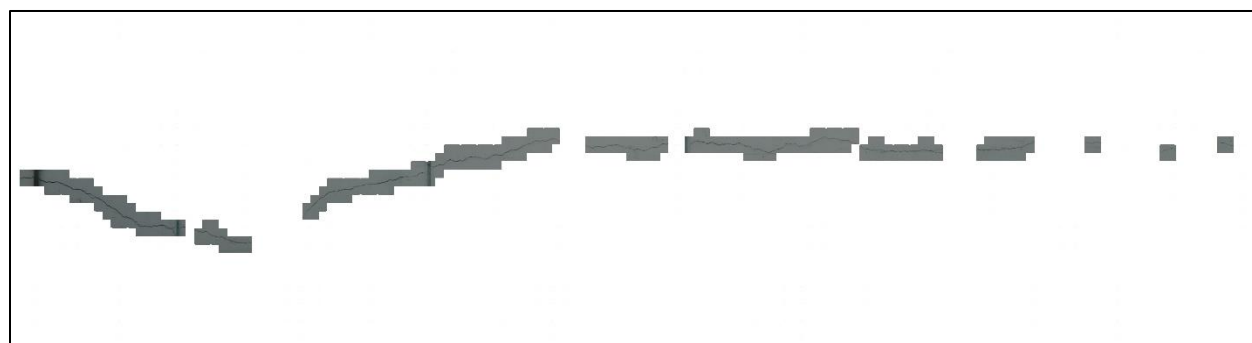
Figure 45- the output image after Figure 40 has been passed through the developed crack detection algorithm.
