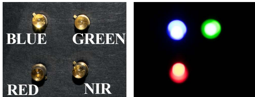
Fig. 2. Shown is the Visible-NIR bands target scene created using 3 visible LEDs and 1 NIR LED. Photos show LEDs off (left) and LEDs on (right). These photos are taken with a Nikon D3300 DSLr visible camera.
