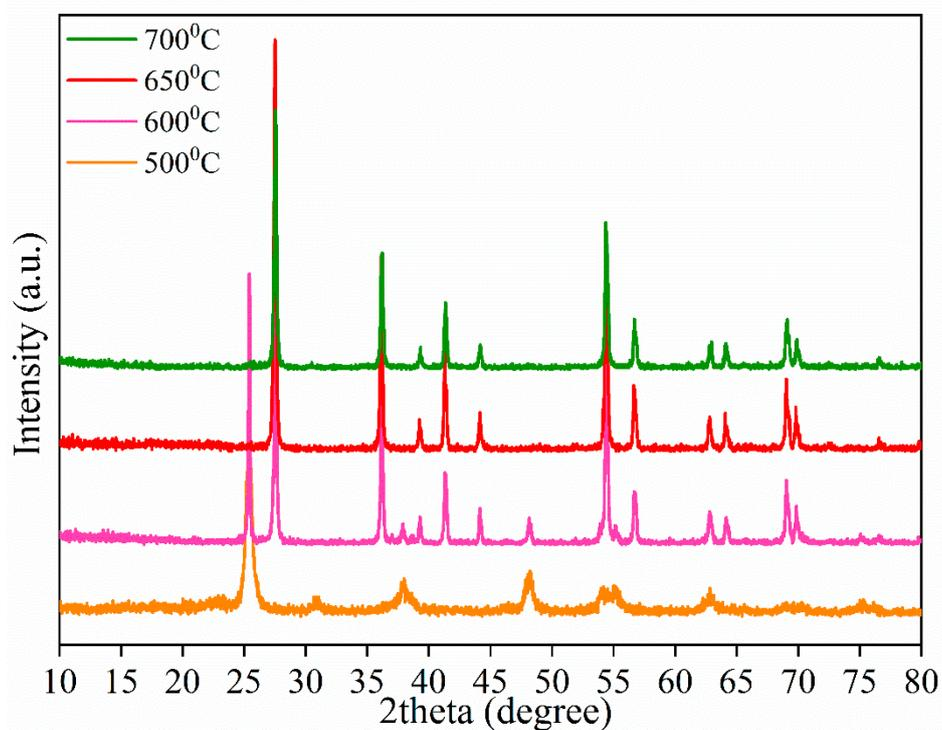
Figure S1. XRD profiles of undoped TiO<sub>2</sub> at different temperatures.
