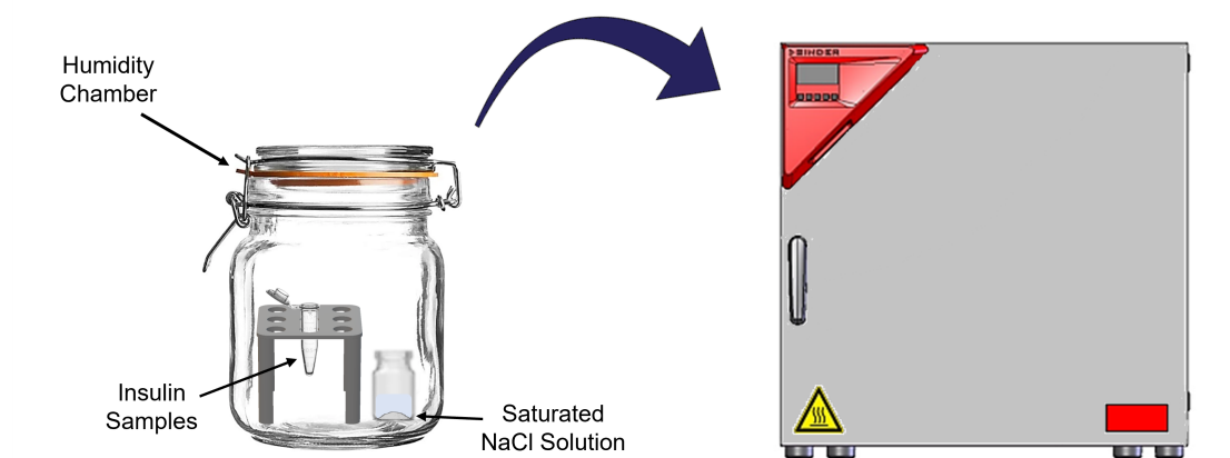
Figure S3.1. Schematic representation of experimental set up. Kilner ® jars were used as bespoke humidity chambers, into which insulin samples and saturated salt solutions were placed. Humidity chambers were then placed in ovens with set temperatures.
