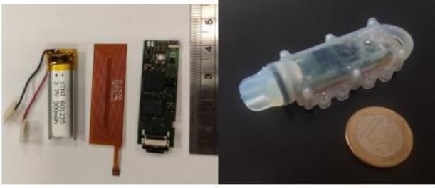
Figure 3. AquaBit seaweed monitoring tag [17].
