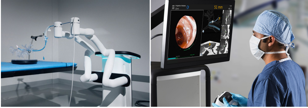
Figure 1.1: The MONARCH™ robotic endoscopy platform (Auris Health Inc., Redwood City, CA) [10], as an example of EMT-guided medical intervention.
