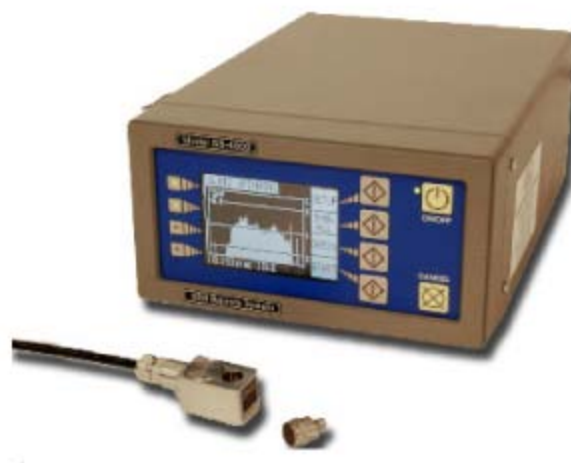
Figure 1.20: Example of an acoustic sensor for grinders
