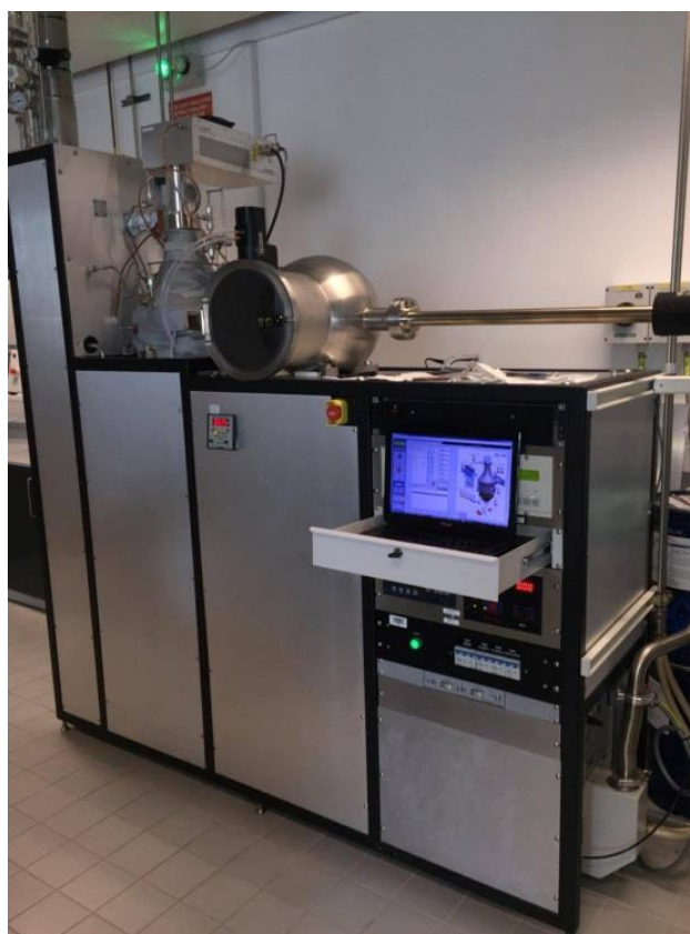
Figure 2.1: The Cambridge Nanotech Fiji 200 ALD deposition system at the Tyndall National Institute
