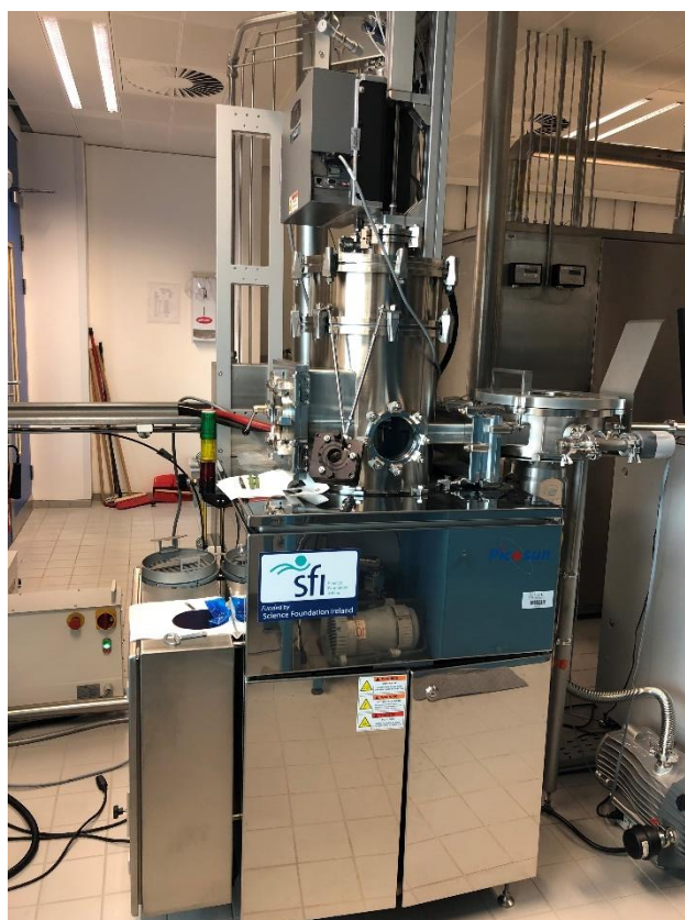
Figure 2.3: The Picosun ™ R200 ALD deposition system at the Tyndall National Institute
