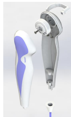
Figure 5.6 Exploded view of SafeTrac handle render in SolidWorks.
