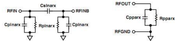
Figure 9. The LNA (left) and PA (right) models
